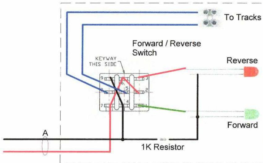
This circuit uses a 3 pole changeover switch. The Positive and Negative (RED & BLACK) are connected to the switch as shown (where they cross each other on the back of the switch ensure they are insulated, as they will create a dead short if they touch each other). The LED indicators are connected as shown with the 1K resistor on the Negative line. If using 12v Filament bulbs the resistor is not required.
